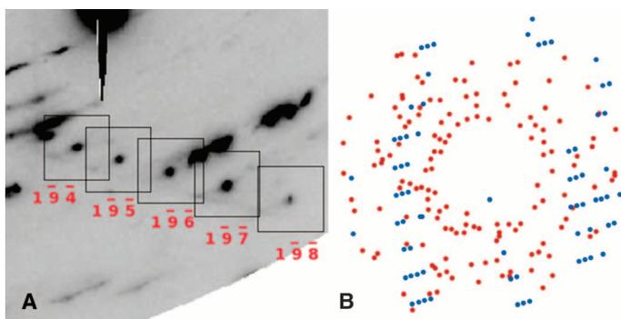
**Fig. 1. Row of reflections of an  $\text{Fe}_5\text{O}_6$  crystal in a multiphase diffraction pattern.** (A) Detail of an x-ray diffraction pattern collected at 18 GPa, highlighting an indexed row of peaks belonging to an  $\text{Fe}_5\text{O}_6$  crystal. (B) In a projection in the reciprocal space of all reflections, those belonging to the  $\text{Fe}_5\text{O}_6$  grain are shown in blue.
