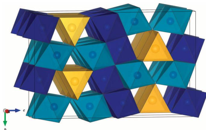
**Fig. 2. The structure of  $\text{Fe}_5\text{O}_6$ .** The trigonal prisms representing the coordination environment of iron in the  $4c$  position are shown in yellow. Layers of edge-sharing coordination octahedra of iron in the  $8f$  positions are shown in two shades of blue representing two non-equivalent crystallographic sites.
