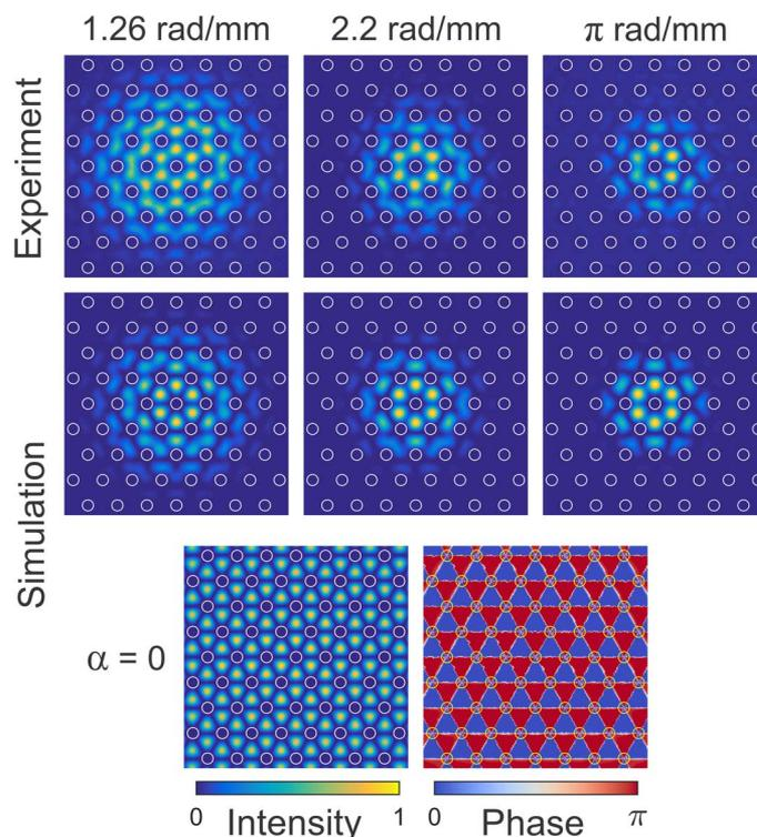
**Fig. 3. Experimental (upper) and calculated (middle) axial Poynting vector distributions at a wavelength of 818 nm for twist rates 1.26, 2.20, and  $\pi$  rad/mm.** The locations of the hollow channels are marked with white circles. The two lower plots show the calculated axial Poynting vector (left) and phase (right) distributions at the bottom of the passband in the untwisted case, when there is no bound mode.
