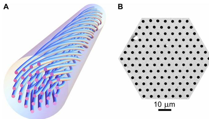
**Fig. 1. The geometry of the twisted coreless PCF.** (A) Schematic of a twisted coreless PCF. The axis of rotation coincides with the hollow channel in the center. (B) Scanning electron micrograph of the microstructure.
