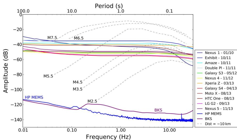
**Fig. 1. Noise floor of the phones.** Noise floors of the smartphones color coded by the phone release date (also shown in the legend as MM/YY). Dashed black lines are typical ground motion amplitudes of earthquakes 10 km from the epicenter for various magnitudes. Noise floor for high-quality MEMS sensor (HP MEMS, blue) and a typical force-balance accelerometer from a regional network (BKS in northern California, purple) are also shown.
