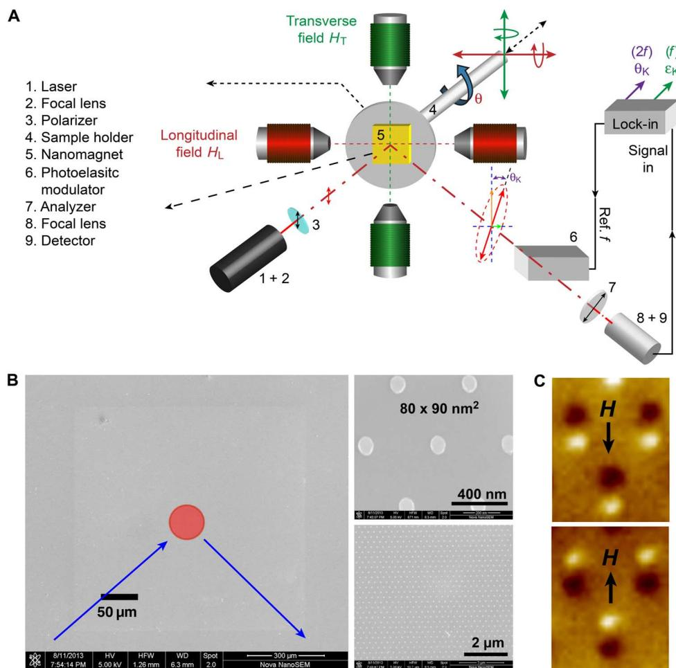
**Fig. 2.** The magneto-optic Kerr microscopy experimental set up. (A) Schematic of the experimental MOKE setup. (B) SEM images of the sample. The circle represents the approximate size of the probe laser spot. (C) MFM images of individual single-domain nanomagnets.
