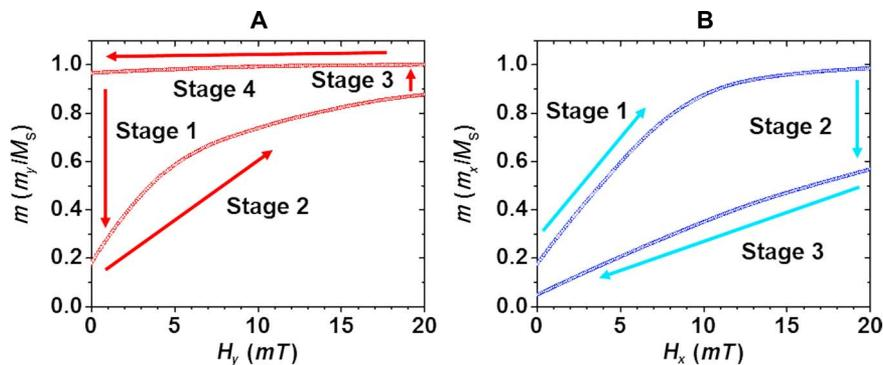
**Fig. 3. The experimental  $m$ - $H$  hysteresis loops of nanomagnets during the reset operation. (A and B) The  $m_y$ - $H_y$  loop (easy axis) (A) and the  $m_x$ - $H_x$  loop (hard axis) (B). The indicated stages correspond to the timing diagram shown in Fig. 1B.**
