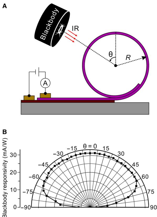
**Fig. 2. Omnidirectional coupling of a rolled-up 3D tubular QWIP device.** (A) Schematic diagram of a 3D tubular QWIP illuminated by the infrared radiation (IR) of a blackbody source with an angle  $\theta$  to the vertical direction. (B) Its blackbody responsivity at various angles.
