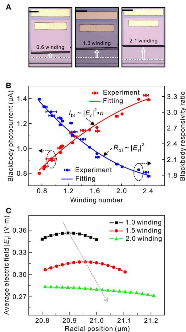
**Fig. 4. Rolled-up 3D tubular QWIPs with different windings.** (A) Optical images of rolled-up 3D tubular QWIPs with 0.6, 1.3, and 2.1 winding, respectively. Scale bar, 200  $\mu\text{m}$ . (B) Blackbody photocurrent and blackbody responsivity ratio as a function of winding numbers with the error bars. (C) Simulated average electric field along the radial direction of the tubular structure with the winding numbers of 1.0, 1.5, and 2.0, respectively.
