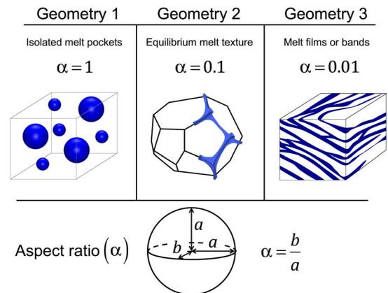
**Fig. 2. Conceptual models of the melt geometry used in these calculations.** Geometry 1 is based on the studies of Berryman (37, 38). Geometry 2 is modified from Takei (11), Mavko (12), and Schmeling (39). Geometry 3 is modified from Holtzman and coworkers (6, 22). The effect of any intermediate geometry on seismic velocities can be modeled by modifying the aspect ratio ( $\alpha$ ) in Eqs. 3 and 4 [see the study of Takei (11) for further discussion of the derivation of  $\alpha$ ].
