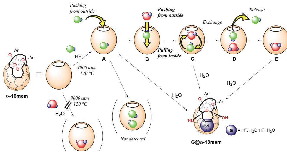
**Fig. 2. Insertion mechanism of HF, H<sub>2</sub>O-HF, and H<sub>2</sub>O into  $\alpha$ -16mem with the synergistic effects of pushing from outside by high-pressure conditions and pulling from inside by attractive interaction of HF with the outer H<sub>2</sub>O.**
