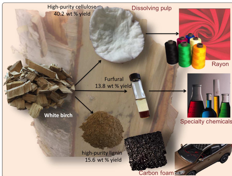
Fig. 1. TriVersa Process. Lignocellulosic biomass can be fractionated into its main components to replace petroleum-derived chemicals used in daily life. Initial composition of white birch (dry weight): hexosan, 45.0 wt %; pentosan, 25.3 wt %; lignin, 21.7 wt %. The yields have been calculated on the basis of our techno-economic analysis.
