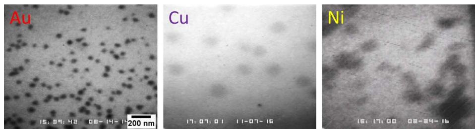
Fig. 4. Electrochemical + radiolytic formation of Au, Cu, and Ni nanocrystals. All growths occur in 0.1 M HCl during linear potential sweeping at 1 mV/s for Au, 5 mV/s for Cu, and 1 mV/s for Ni. The measured onset potentials are shown in table S1 and other electrochemical parameters are shown in fig. S7. All images are obtained at the same field of view.
