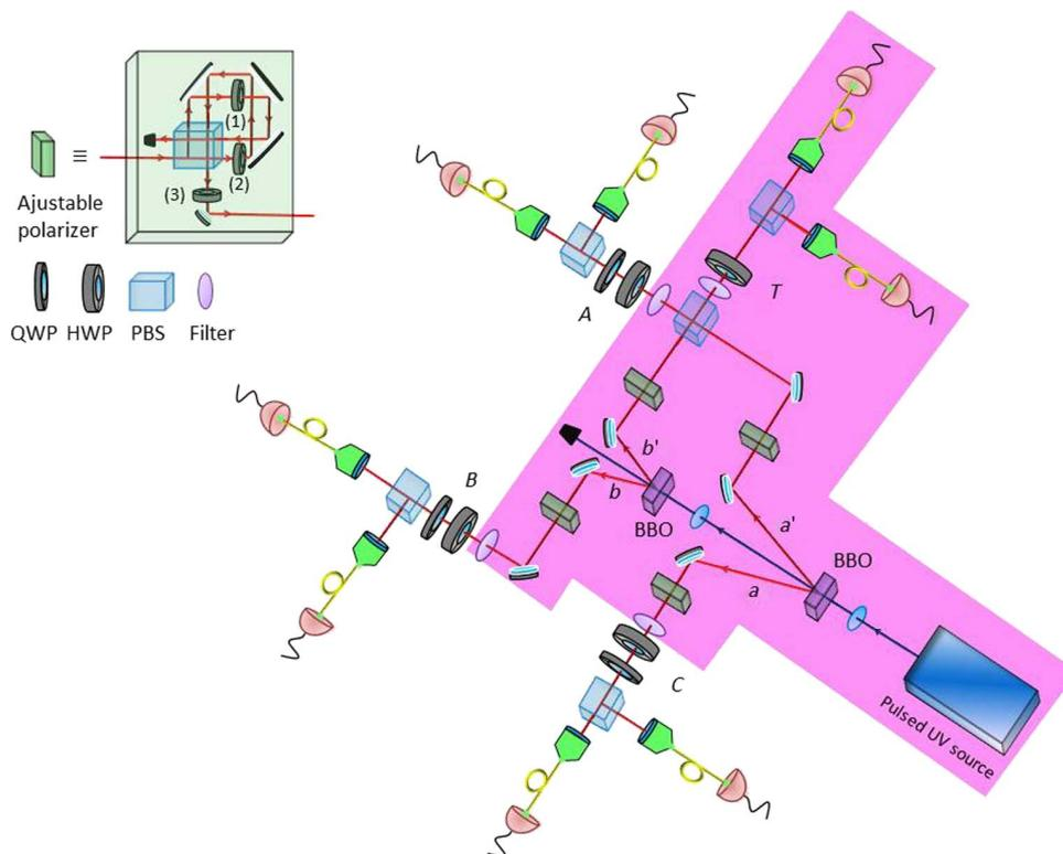
**Fig. 6. Experimental setup for the generation of three-qubit polarization bound entangled state.** The colored area represents the state preparation. See Methods for more details. QWP, quarter-wave plate; HWP, half-wave plate; PBS, polarizing beam splitter; BBO,  $\beta$ -barium borate; UV, ultraviolet.
