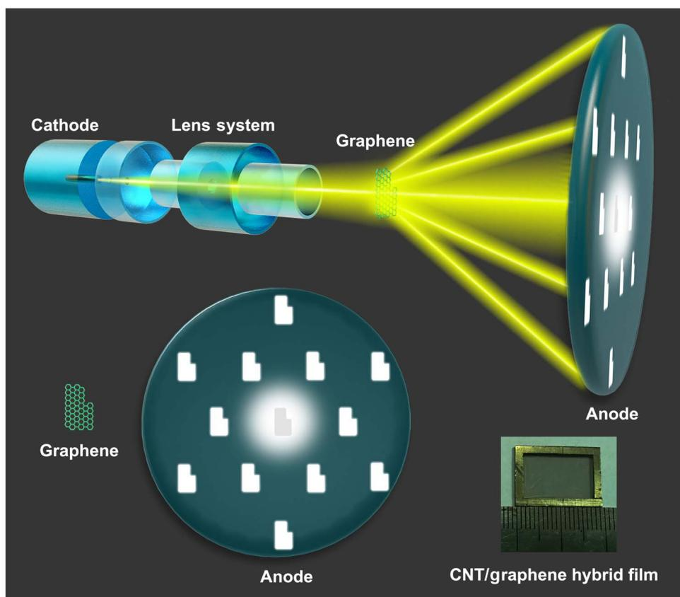
**Fig. 1. Schematic of the low-energy transmission electron diffraction system.** Thermionic cathode, lens system, graphene sample, SACNT film sample support (not shown), and phosphor anode. The lens system can be tuned to generate electron beams of variable size (from 400  $\mu\text{m}$  to 1 cm in diameter). The front view of the graphene sample and anode is shown. The inset at the bottom right shows a photograph of a CNT/graphene hybrid film (CGF) more than 1.6 cm long.
