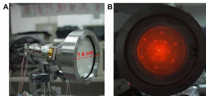
**Fig. 5. A compact instrument for transmission electron diffraction and imaging.** (A) Photograph of the compact instrument. (B) Transmission electron diffraction pattern of polycrystalline graphene acquired by using the compact instrument. With the help of an MCP, the diffraction spots of adsorbates and graphene can be seen at normal illumination.
