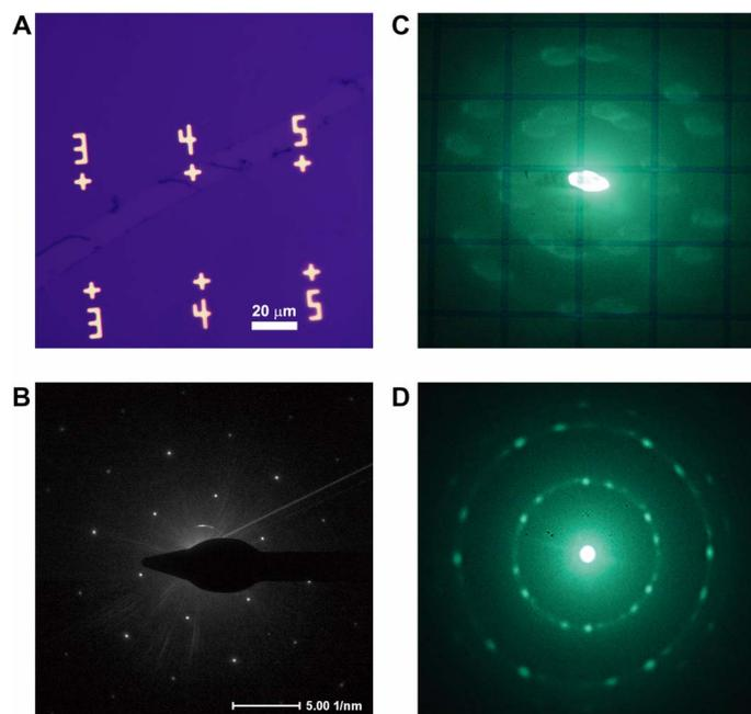
**Fig. 3. Transmission electron diffraction and imaging of large-area continuous polycrystalline graphene.** (A) Optical image of transferred large-area continuous polycrystalline graphene on silicon substrate (with SiO<sub>2</sub> layer). (B) SAED pattern of polycrystalline graphene (200 keV), with an aperture size of 100 nm. (C) Transmission electron diffracted image of large-area continuous polycrystalline graphene.
