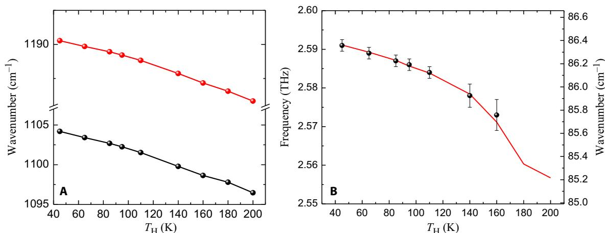
**Fig. 2. Frequency tuning.** Dependence of mid-IR pump frequencies (A) and THz difference frequency (B) of the THz DFG-QCL on the  $T_H$ . The device was operated in pulsed mode, as described in the main text. The solid line in (B) represents the frequency difference of the two mid-IR peaks as extracted from (A), and the round symbols with error bars indicate the experimentally measured THz peak positions.
