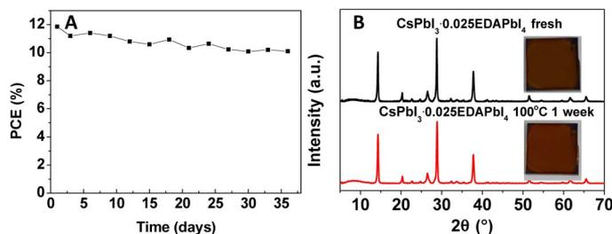
**Fig. 5. Stability test of CsPbI<sub>3</sub>-0.025EDAPbI<sub>4</sub>-based devices and films. (A)** PCE of the champion PSC fabricated from CsPbI<sub>3</sub>-0.025EDAPbI<sub>4</sub> as a function of storage time in a dark dry box. **(B)** XRD pattern and images of the CsPbI<sub>3</sub>-0.025EDAPbI<sub>4</sub> film heated at 100°C in a dry box for 1 week.
