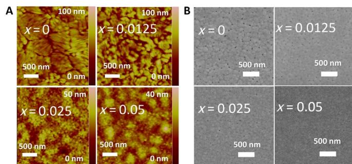
**Fig. 3. Effect of EDAPbI<sub>4</sub> on the evolution of morphology of CsPbI<sub>3</sub>:xEDAPbI<sub>4</sub>.** (A) AFM and (B) SEM images of perovskite films obtained from the CsPbI<sub>3</sub>:xEDAPbI<sub>4</sub> additive precursor ( $x = 0, 0.0125, 0.025,$  and  $0.05$ ).
