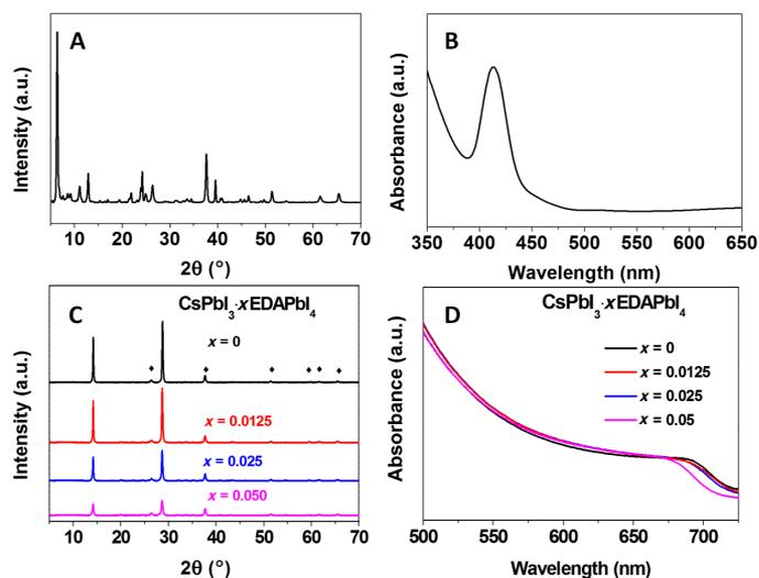
**Fig. 2. Structural characterization and spectroscopic study of EDAPbI<sub>4</sub> and CsPbI<sub>3</sub>·xEDAPbI<sub>4</sub> films.** (A) XRD pattern and (B) UV-vis spectrum of EDAPbI<sub>4</sub> films. (C) XRD patterns and (D) UV-vis absorption spectra of CsPbI<sub>3</sub>·xEDAPbI<sub>4</sub> ( $x = 0$  to 0.05) perovskites.
