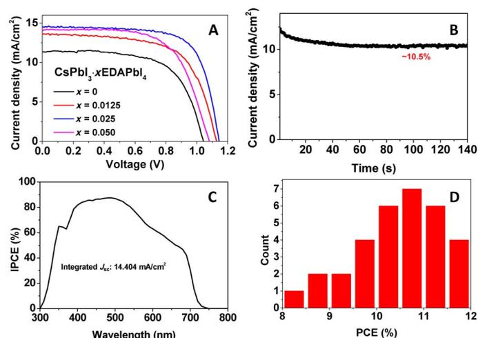
**Fig. 4. Device characteristics for CsPbI<sub>3</sub>:xEDAPbI<sub>4</sub> films.** (A) Typical  $J$ - $V$  curves of CsPbI<sub>3</sub>:xEDAPbI<sub>4</sub> PSCs. (B) Stable current output at the maximum point of the champion CsPbI<sub>3</sub>:0.025EDAPbI<sub>4</sub> PSC. (C) IPCE of the best solar cell based on the CsPbI<sub>3</sub>:0.025EDAPbI<sub>4</sub> perovskite. (D) Histogram of device efficiencies of CsPbI<sub>3</sub>:0.025EDAPbI<sub>4</sub> PSCs based on 32 cells from three batches.
