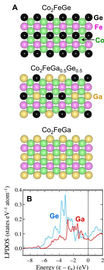
**Fig. 5. Effects of Ga substitution for Ge of  $Co_2FeGe$ .** (A) Schematic illustration of (110) surfaces for  $Co_2FeGe$ ,  $Co_2FeGa_{0.5}Ge_{0.5}$ , and  $Co_2FeGa$ . (B) Local partial DOSs (LPDOSs) of Ge at  $Co_2FeGe(110)$  (blue) and Ga at  $Co_2FeGa(110)$  (red) surfaces.
