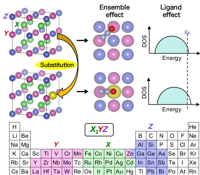
**Fig. 1. Concept of this study.** Effects of elemental substitution are schematically illustrated with the Heusler alloy's crystal structure (L21-type  $X_2YZ$ ) (2). Periodic table represents typical elements consisting of X, Y, and Z (color painted). Other elements such as lanthanoids and those in groups 1 and 2 are also possible components of Heusler alloys [see (6)].
