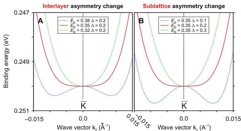
**Fig. 3. Interlayer/sublattice asymmetry.** Demonstration of the possibility of transforming the flat band electronic structure into a band with either positive or negative effective mass by changing (A) the interlayer asymmetry and (B) the sublattice asymmetry of the bottom layer. The calculation is based on the Hamiltonian  $H_2$ .
