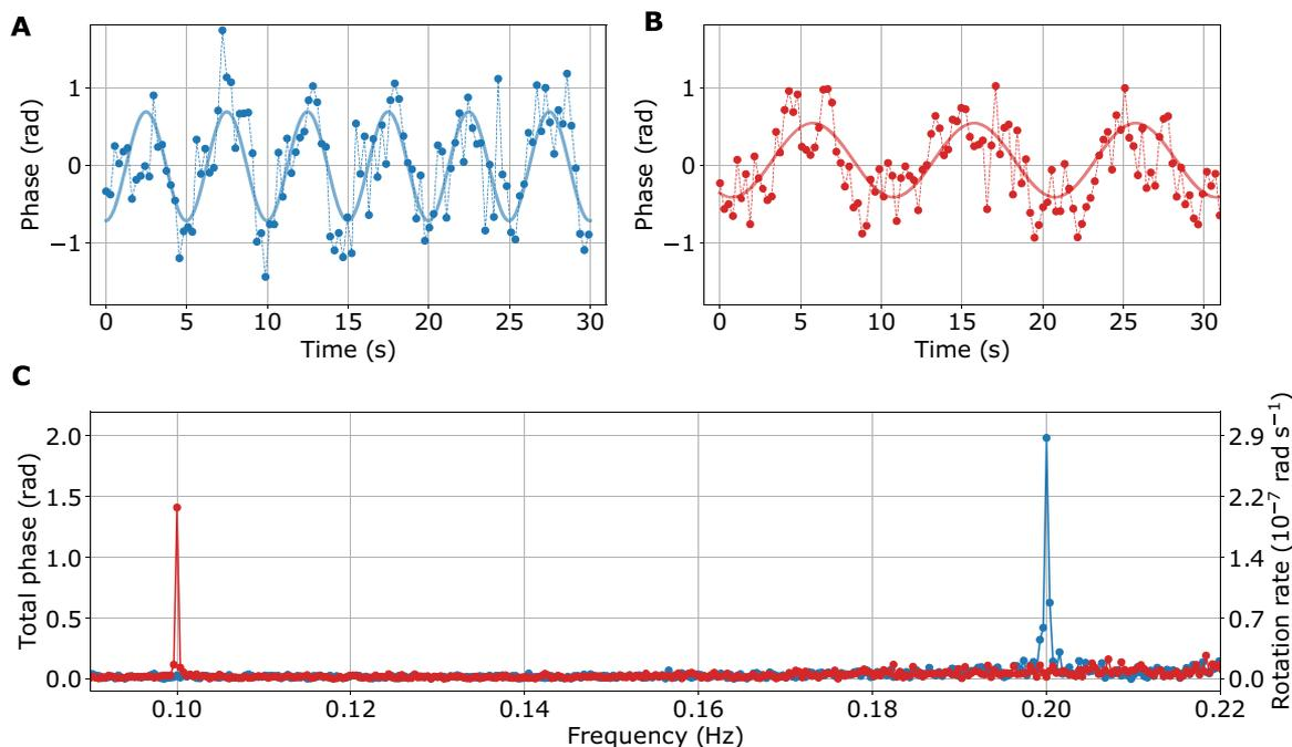
**Fig. 4. Measurement of dynamic rotation rates.** Atom interferometer phase deduced from the transition probability, for rotation rate modulations of 5-s period (A) and 10-s period (B). Plain line, sinusoidal fit to guide the eye. (C) Fourier analysis of the total rotation rate signal, with a frequency resolution of 0.37 mHz.
