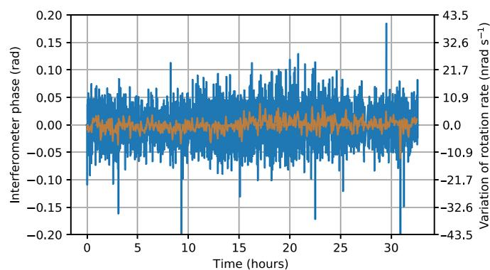
**Fig. 2. Rotation rate measurement during 32.5 hours.** In the blue (orange) trace, each data point is the average over segments of 26.7 s (267 s) of raw inertial phase measurements. The right axis translates inertial phase to rotation rate using the scale factor of the gyroscope to stationary Earth rotation (from Eq. 2).
