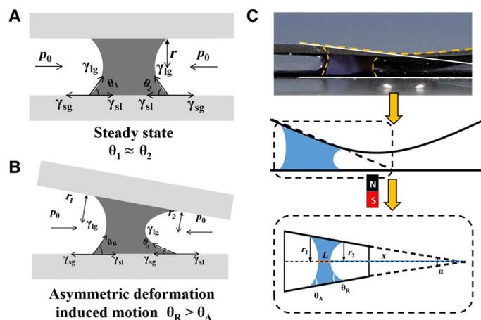
**Fig. 4. Mechanism of the magnetic-controlled liquid transport behavior.** Menisci formed by a liquid drop in an MTMA. (A) Steady state. (B) Conditions for droplet motion induced by the tube asymmetric deformation. (C) Snapshot of a droplet in its transport process and the correspondence between the true actuator and the simplified model.
