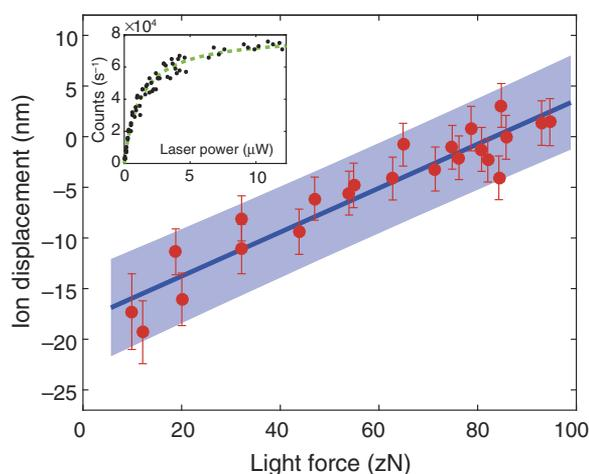
**Fig. 4. Light force detection with a single ion.** Ion displacement as a function of the light force (red dots) and linear fit to experimental data (blue line). The shaded region shows the 95% confidence level for linear fit to experimental data. Inset: Photons scattered by the ion as a function of the laser power. The green dashed line is the fitted curve from Eq. 1, scaled by the detection efficiency, used for calculating the saturation parameter  $s$  as a function of the laser power.
