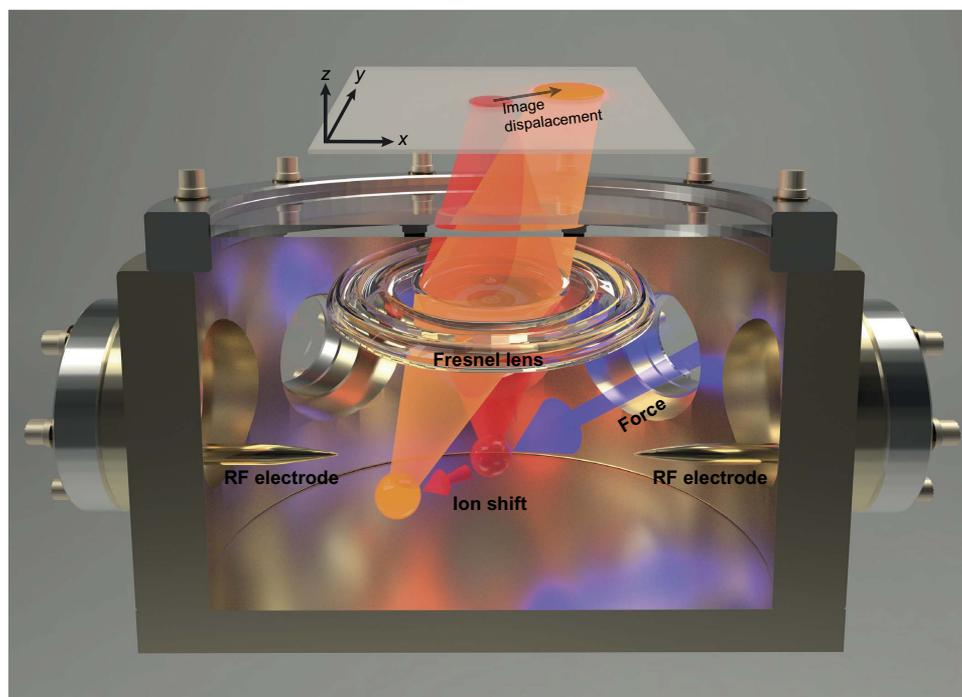
**Fig. 1. Experimental configuration.** An externally applied force (purple arrow) displaces a trapped  $^{174}\text{Yb}^+$  ion. The image formed by the phase Fresnel lens is shifted in two dimensions. Displacement along the focal axis alters the image spot size. For clarity, illustrated trap dimensions are not to scale. RF electrode needle spacing, 300  $\mu\text{m}$ ; lens focal length, 3 mm.
