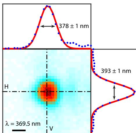
**Fig. 2. Ion image.** Wavelength-scale ion image with Gaussian fitting and FWHM sizes for the horizontal (H) and vertical (V) slices.
