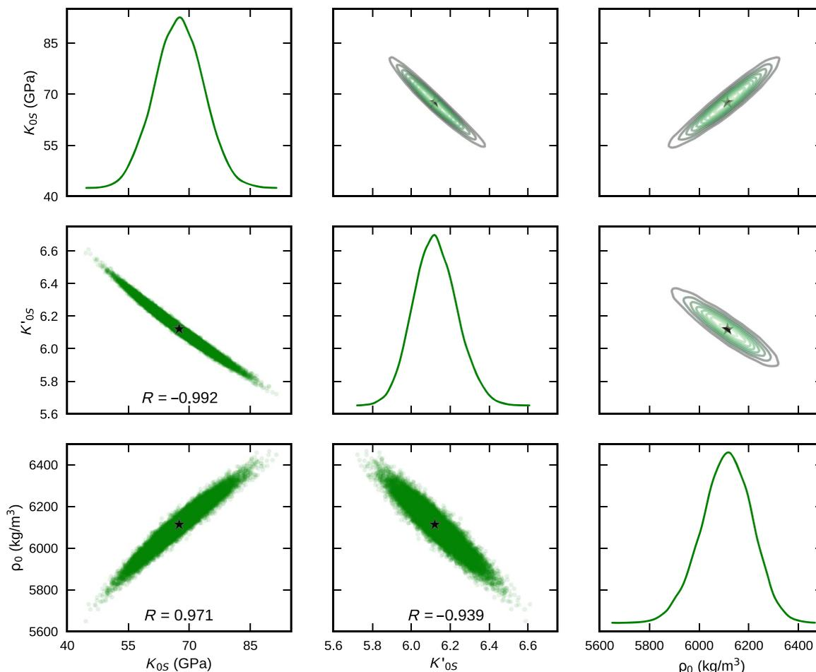
**Fig. 1. Vinet EoS parameter posterior distributions and trade-offs.**  $\rho_0$  is presented using the fixed molar mass of 0.05 kg and inverted molar volume. The black stars show the median values used for the EPOC-Vinet model in Fig. 2. Numbers on the lower left panels indicate correlation coefficients between the parameters in question.
