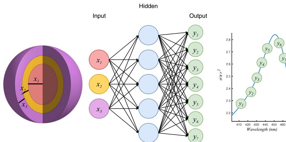
**Fig. 1.** The NN architecture has as its inputs the thickness of each shell of the nanoparticle, and as its output the scattering cross section at different wavelengths of the scattering spectrum. Our actual NN has four hidden layers.
