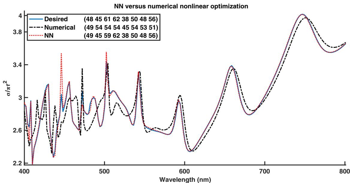
**Fig. 3. Inverse design for an eight-shell nanoparticle.** The legend gives the dimensions of the particle, and the blue is the desired spectrum. The NN is seen to solve the inverse design much more accurately.
