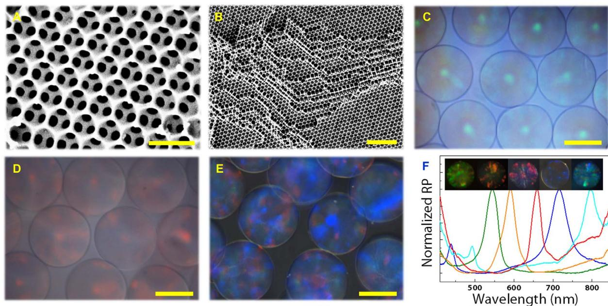
**Fig. 2. SEM images and metalloscope images of the inverse opal particles.** (A) The surface and (B) the inner side of an inverse opal particle with a higher concentration of the cross-linker. (C to E) Reflection images of the green, red, and blue inverse opal particles. (F) Reflection peaks and reflection images of five different inverse opal particles. RP, reflective percent. Scale bars, 500 nm (A), 2  $\mu\text{m}$  (B), and 100  $\mu\text{m}$  (C to E).
