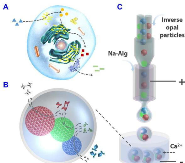
**Fig. 1. Schematics of the preparation of the bioinspired microcapsules.** (A) Schematic of the enzyme cascade reaction in a cell. (B) Schematic of the enzyme cascade reaction in the microcapsule encapsulated with enzyme-immobilized inverse opal particles. (C) Schematic of the microcapsule generation process with the microfluidic electrospay.
