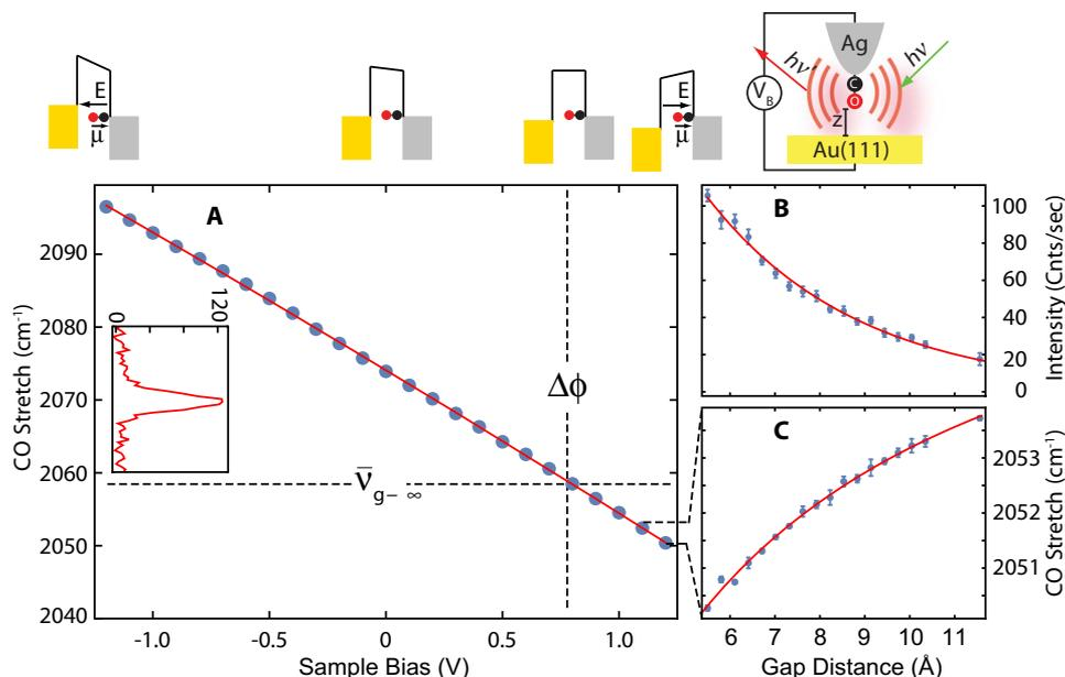
**Fig. 1. Calibration of the molecular electrometer.** (A) Bias dependence with a gap fixed at  $5.5 \text{ \AA}$  (set at  $0.1 \text{ nA}$ ,  $+1.2 \text{ V}$ ). The inset shows the CO line spectrum. (B) Gap dependence of Raman intensity and (C) C–O stretching frequency. All data are recorded with an excitation at  $\lambda = 634 \text{ nm}$  and an incident intensity of  $\sim 5 \text{ \mu W}/\mu\text{m}^2$ .
