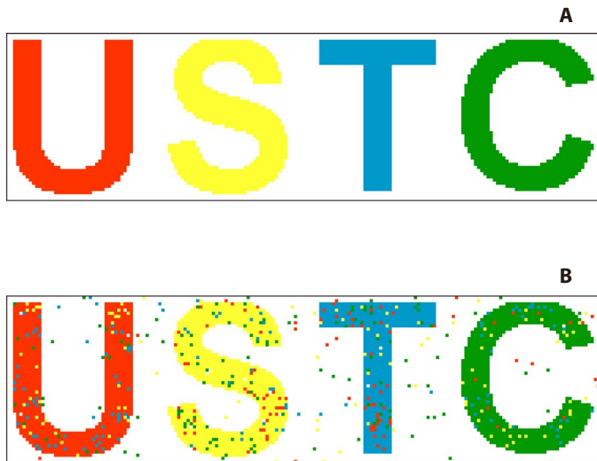
Fig. 3. Transmit a real five-color image using encoded information. Red spots are encoded to \Psi_{11} , yellow spots are encoded to \Psi_{12} , blue spots are encoded to \Psi_{13} , green spots are encoded to \Psi_{14} , and white spots are encoded to \Psi_{23} . (A) Original five-color 53 \times 188 pixel image. (B) Image received using SDC. The calculated fidelity is 0.952.
