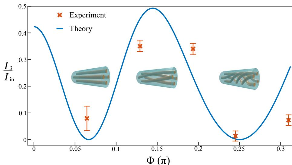
**Fig. 2. Dependence of optical tunneling dynamics on the AB phase.** Normalized light intensity at the output of core #3 for different values of the AB phase  $\phi$  (as induced by different twist rates). In all cases, core #1 is excited at the input with CW laser light at  $\lambda = 1550$  nm. Theoretical results corresponding to the same set of parameters are also provided for comparison. At  $\phi = \pi/4$ , the third core always remains dark, indicating AB tunneling suppression.
