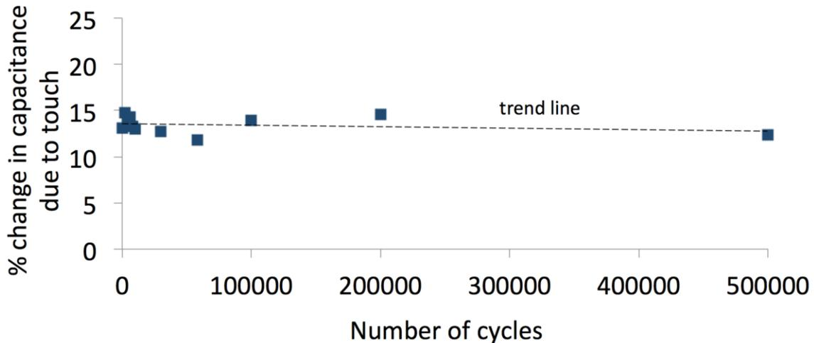
**fig. S5. Plot showing change in capacitance in percentage due to a touch after cycles of 10% strain, followed by a buckling with a radius of curvature of 16 mm.**
