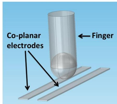
**fig. S1. Coplanar electrode capacitor with a finger.**
