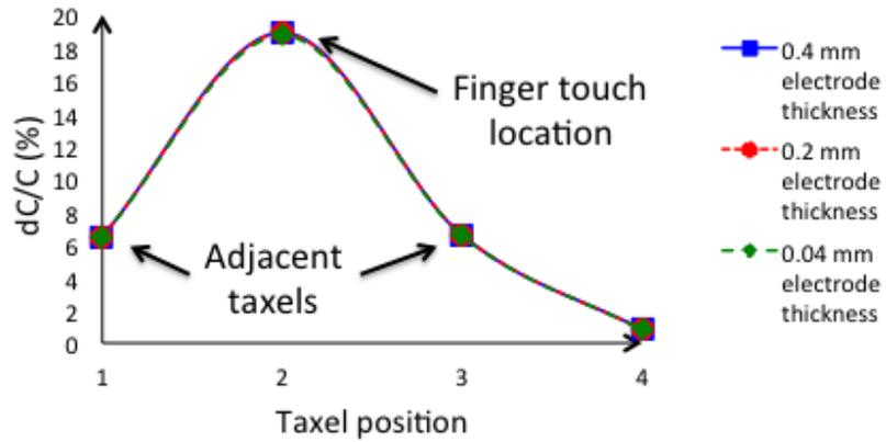
**fig. S3. Effect of scaling on change in capacitance along a row due to a touch at a single taxel.**
