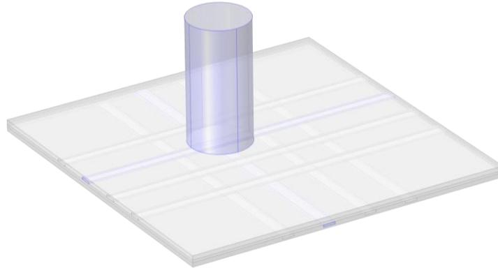
**fig. S2. Finger on an array of capacitive sensors.**
