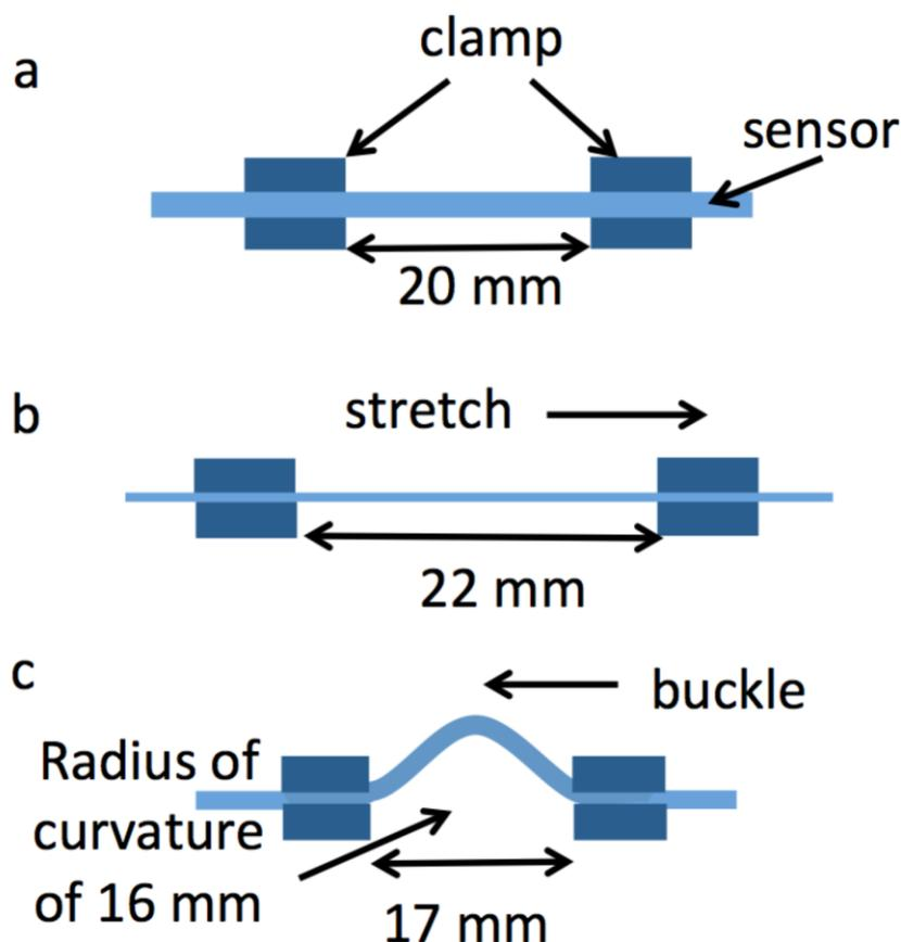
**fig. S4. Steps of mechanical test.** (a) Steady state (b) stretched by 10% strain (c) buckled with an approximate radius of curvature 16 mm.
