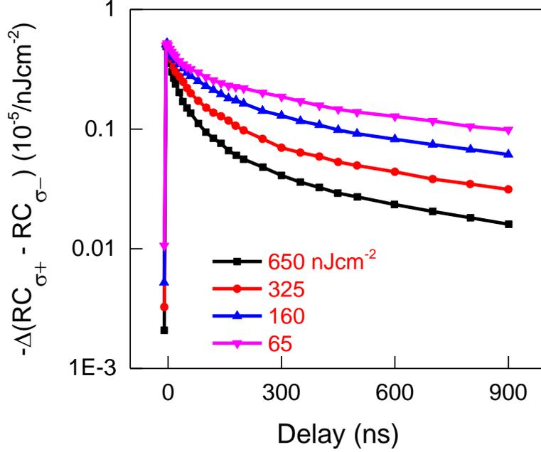
**fig. S1. CD signal of the heterostructure at 10 K with different pump fluence from 65 to 650 nJ cm<sup>-2</sup>.** The initial fast decay components depend sensitively on the pump fluence, which is dominated by interactions between photo-excited carriers.
