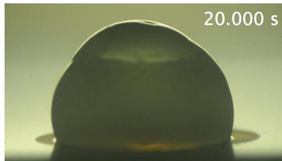
**Movie S1. Droplet freezing.** Freezing of a  $40\text{-}\mu\text{l}$  droplet on the photo-thermal trap, supercooled to  $-17\text{ }^{\circ}\text{C}$  at an ambient temperature of approximately  $-20\text{ }^{\circ}\text{C}$ . Time sequence is shown from 10 seconds before to 50 seconds after recalescence. The video is shown in real-time (recorded at 24 Hz and compressed to 8 Hz).
