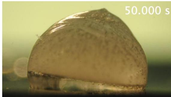
**Movie S2. Droplet melting.** Melting of a 40- $\mu\text{l}$  (frozen) droplet on the photo-thermal trap, at an ambient temperature of  $-25\text{ }^{\circ}\text{C}$  and  $1.8\text{ kW/m}^2$  illumination starting at  $t = 0$ . Time sequence is shown from 5 seconds before to 120 seconds after start of illumination. The video is shown in real-time (recorded at 24 Hz and compressed to 8 Hz).
