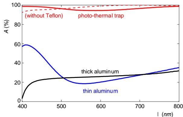
**Fig. S1. Sample absorptivity.** Absorptivity (%) as a function of wavelength (400-800 nm) for the photo-thermal trap coated with cermet (red) *versus* uncoated aluminum (thin and thick sample: blue and black, respectively). All surfaces are coated with Teflon for hydrophobicity, except for the photo-thermal trap reference case indicated by the red dashed line.
