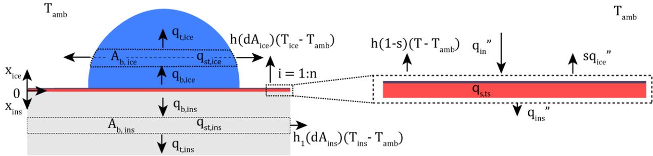
**Fig. S2. Control volume approach to determine the transient temperature evolution of the metal spreader upon illumination.** Control volumes are taken in the ice and insulation to find their respective temperature gradients, while the metal spreader is at homogeneous temperature.
