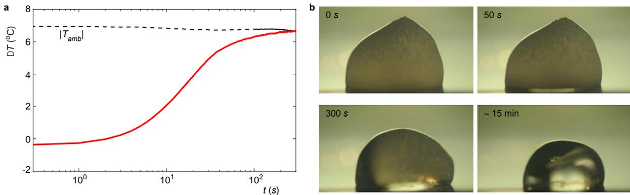
**Fig. S3. Substrate under direct shear flow.** **a** Heating curve (red) for  $1\text{ kW/m}^2$  illumination of the photo-thermal trap at ambient temperature of  $-7\text{ }^{\circ}\text{C}$  (black dashed), and a shear flow leading to increased heat transfer coefficient  $h \sim 70\text{ W/m}^2/\text{K}$ . **b** Snapshots show intermediate steps in the progression of melting on the photo-thermal trap.
