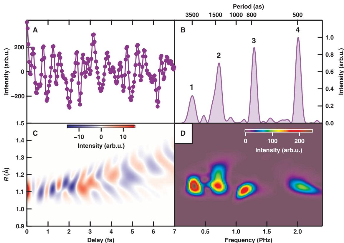
**Fig. 2. Attosecond electron responses in the pump-probe measurement.** (A) Temporal evolution of fragment ion intensity at  $E = 0.2$  eV. (B) Fourier power spectrum of (A). (C) Numerical simulation of the nuclear correlation function  $\text{Re} \left[ \sum_{i<j} \Psi_i^*(R, \Delta t) \Psi_j(R, \Delta t) \right]$  composed of four pairs of electronic states. (D) Fourier power spectrogram of (C).
