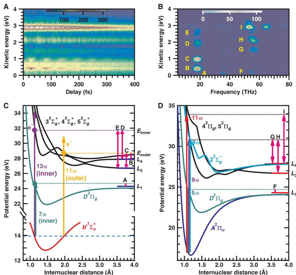
**Fig. 3. Temporal evolution of VWP for assigning EWP.** (A) Delay-dependent KE distribution of  $N^+$ . (B) Frequency-KE spectrogram of (A). (C) Probe scheme of the VWP prepared in the  $b^1\Sigma_u^+$  state. (D) Probe scheme of the VWP prepared in the  $A^2\Pi_u$  state.
