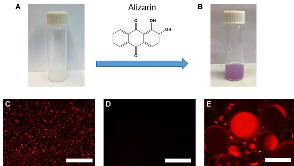
**Fig. 4. Visualization of HA NP pickup using alizarin-labeled NPs.** (A) Commercial HA NP suspended in ethanol before staining. (B) Alizarin-labeled HA NPs suspended in ethanol. (C) Fluorescence micrograph of alizarin-labeled HA NP-coated substrate. (D) Same substrate after HA NP pickup using polymer 4-stabilized droplets. (E) Fluorescence micrograph of polymer 4-stabilized droplets following NP pickup. Scale bars (C to E), 500  $\mu\text{m}$ .
