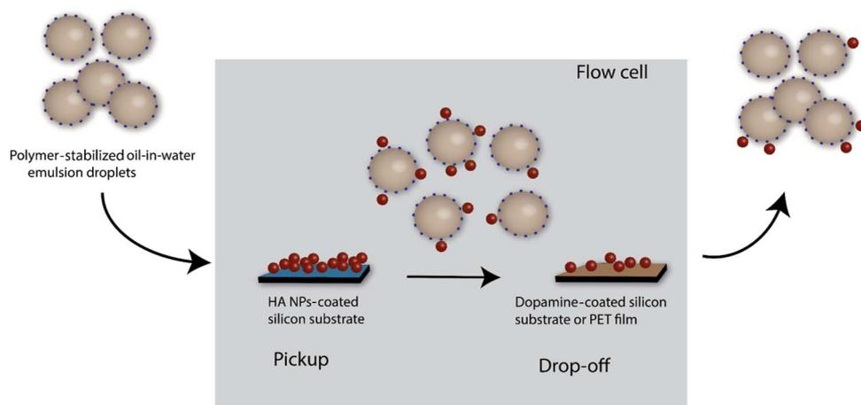
**Fig. 5. Illustration of HA NP pickup and drop-off.** The oil-in-water emulsion droplets stabilized by polymer **4** pick up HA NPs from the Si substrate and then drop them off downstream on the PDA-coated Si substrate or PET film.
