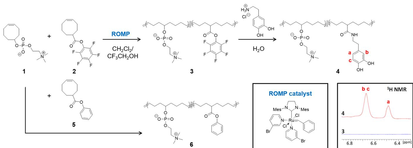
**Fig. 2. Synthesis of polymers 3, 4, and 6. (Insets)** Chemical structure of the 3-bromopyridine-substituted Grubbs catalyst and the aromatic region of the  $^1\text{H}$  NMR spectra of polymers 3 and 4.
