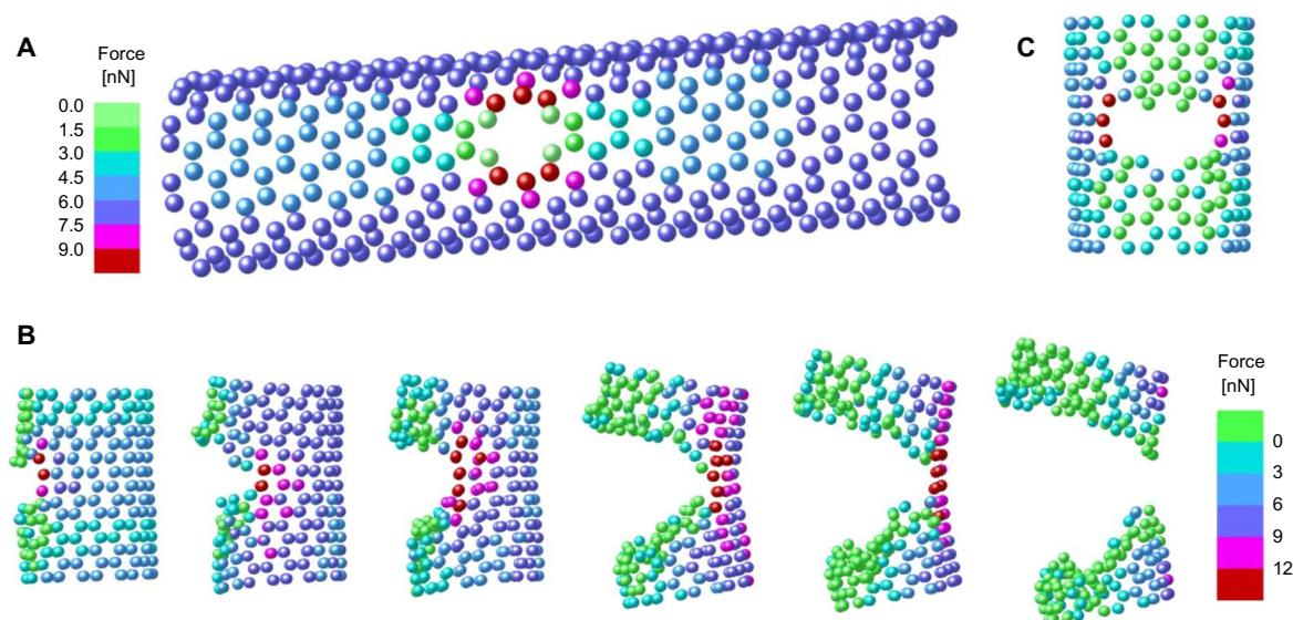
**Fig. 3. High stresses around a defect lead to crack propagation.** (A) Nonuniform stress distribution in an armchair SWNT containing a two-atom vacancy defect [Fig. 1B(c)], under tensile loading at 10% strain, expressed in terms of atom forces in the loading direction. The highest stressed atoms are colored red. (B) Spontaneous crack propagation at a fixed strain of 11%. The loading direction is vertical, and the crack is viewed from the side. (C) Atom forces around a crack (front view).
