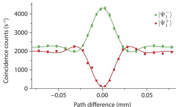
**Fig. 2. Photon coincidence counts measured as a function of the path length difference.** The red points denote input states  $|\Psi_1^+\rangle$ , and the green points denote input states  $|\Psi_1^-\rangle$ . We observe a HOM interference dip/peak when the path length difference is equal to zero. The data points shown are the average of 20 readings. A Gaussian function multiplied by a sinc function was fitted to the data and is shown as solid curves.
