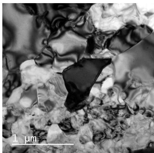
**Fig. 2. Transmission electron micrograph of an aggregate of (Mg,Fe)SiO<sub>3</sub> tetragonal majorite in Tenham.** The ATEM sample consists of monomineralic aggregates of euhedral or subhedral grains. No interstitial phases are present among the majorite grains.
