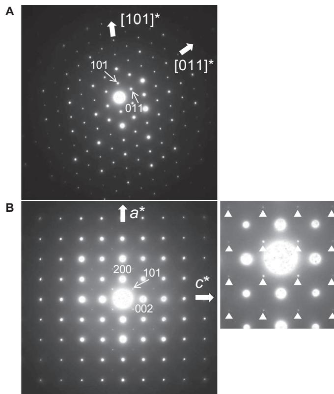
**Fig. 3. SAED patterns from single crystals of (Mg,Fe)SiO<sub>3</sub> tetragonal majorite.** (A) Along the  $[1\bar{1}1]$  zone axis. (B) Along the  $[010]$  zone axis. Weak  $\{h0l\}$  reflections, where both  $h$  and  $l$  are odd [indicated by triangles in the magnified pattern (right)] are diagnostic reflections for the tetragonal  $I4_1/a$  symmetry.
