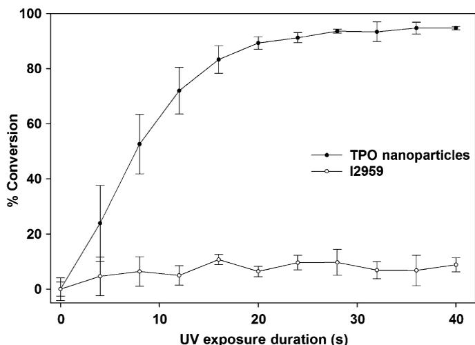
**Fig. 3. Polymerization kinetics.** Percentage of conversion of vinyl bonds calculated using aqueous acrylamide solutions with TPO nanoparticles and I2959 at  $988\text{ cm}^{-1}$  (assigned to the out-of-plane bending mode of the  $=\text{C}-\text{H}$  unit) normalized to the  $\text{C}=\text{O}$  stretching peak at  $1654\text{ cm}^{-1}$  as an internal standard at varying durations of UV (395-nm) exposure.
