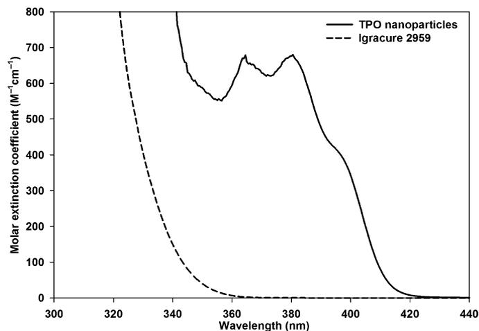
**Fig. 2. Molar extinction coefficient of TPO nanoparticles.** Molar extinction coefficients of the TPO nanoparticles (solid line) and I2959 (dashed line) obtained by measuring the absorbance of 4 mM aqueous solutions.
