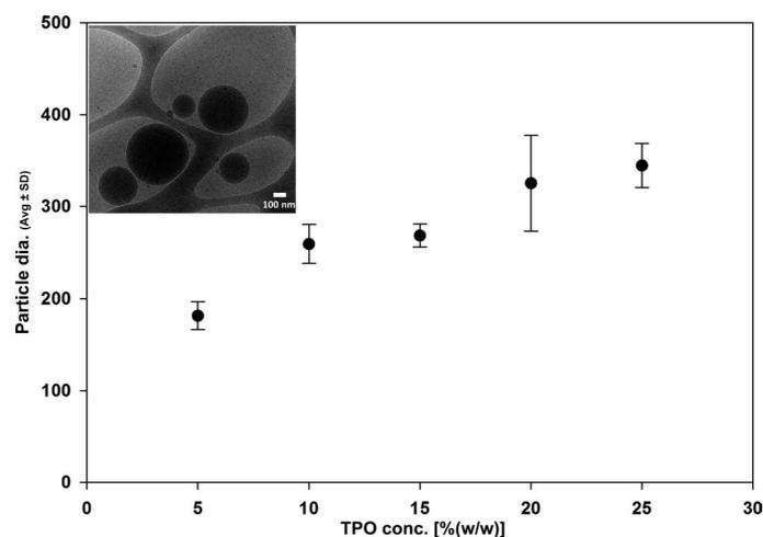
**Fig. 1. TPO nanoparticle size.** Average (Avg) particle size of an aqueous dispersion of 0.1% (w/w) powder containing TPO nanoparticles obtained from microemulsions with various concentrations of TPO. Inset: Cryo-TEM image of an aqueous dispersion [0.1% (w/w)] of powder containing 25% (w/w) TPO.
