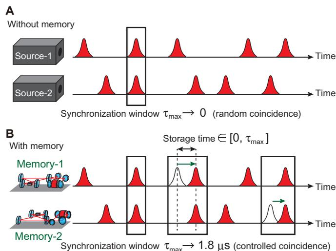
**Fig. 1. Synchronization of optical photons.** (A) Independent statistical photon sources without memories. (B) Independent photon sources with memories.  $\tau_{\max}$  the maximum storage time. In principle, the synchronization window could be further increased beyond 1.8  $\mu\text{s}$ ; however, in our present performance of memories, this would be at the expense of the negativity of the Wigner function.
