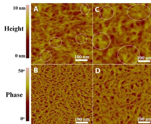
**Fig. 6. AFM images of DPPTTT and DPPTTT-NMe<sub>4</sub>I.** (A to D) AFM height and phase images of the neat DPPTTT thin film (A and B) and the DPPTTT-NMe<sub>4</sub>I thin film at a molar ratio of 30:1 (C and D). The circles in (C) highlight the formation of more connected and larger fiber aggregates within the DPPTTT-NMe<sub>4</sub>I thin film in comparison with those marked by circles in (A) for the neat DPPTTT thin film.
