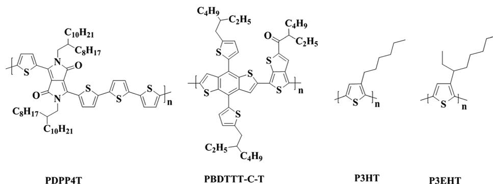
**Fig. 9. Chemical structures of PDPP4T, PBDTTT-C-T, P3HT, and P3EHT.**
