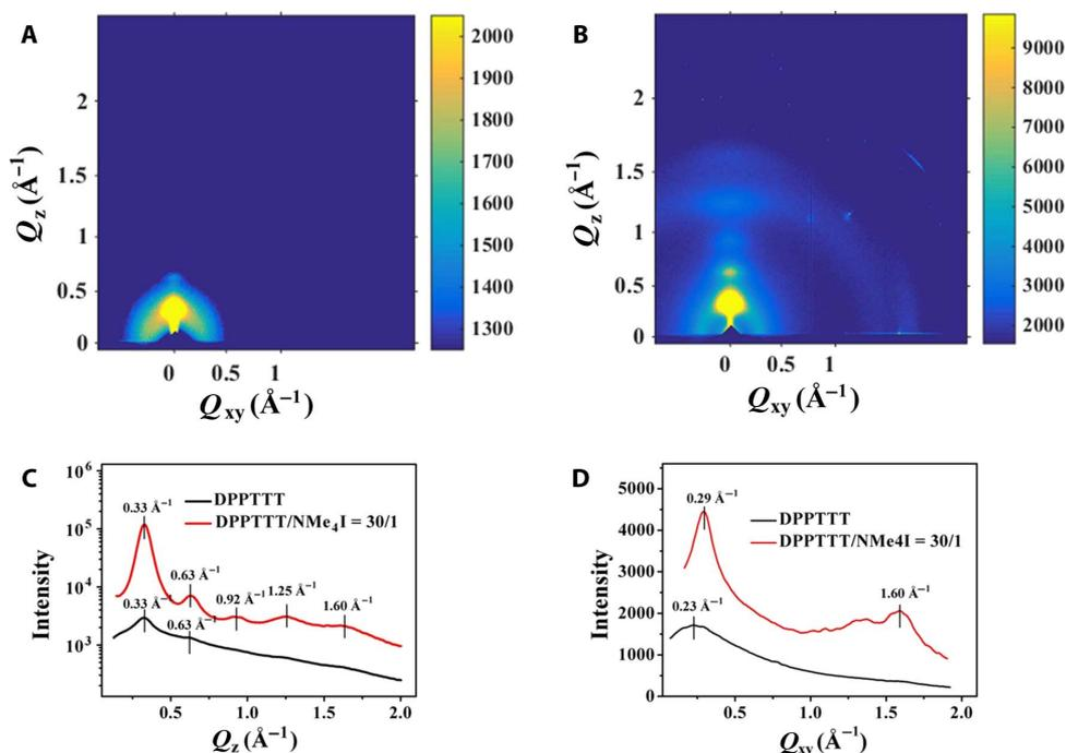
**Fig. 7.** GIWAXS patterns of DPPTTT and DPPTTT-NMe $_4$ I thin films. (A and B) 2D GIWAXS images of DPPTTT (A) and DPPTTT-NMe $_4$ I (B) at a molar ratio of 30:1. (C) Out-of-plane linecuts of 2D GIWAXS of DPPTTT and DPPTTT-NMe $_4$ I at a molar ratio of 30:1. (D) In-plane linecuts of 2D GIWAXS of DPPTTT-NMe $_4$ I at a molar ratio of 30:1.
