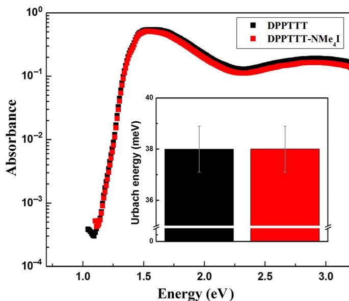
**Fig. 5. PDS spectra of DPPTTT and DPPTTT-NMe<sub>4</sub>I thin films.** PDS spectra of thin films of DPPTTT and DPPTTT-NMe<sub>4</sub>I at a molar ratio of 30:1. The inset shows the respective Urbach energies.
