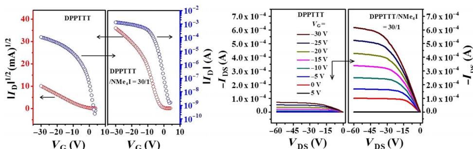
**Fig. 2. OFET characteristics for DPPTTT and DPPTTT-NMe<sub>4</sub>I.** Transfer ( $V_{\text{DS}} = -60 \text{ V}$ ) and output characteristics of neat DPPTTT and DPPTTT-NMe<sub>4</sub>I at a molar ratio of 30:1; the transistor channel width ( $W$ ) and channel length ( $L$ ) were 8800 and  $80 \mu\text{m}$ , respectively.
