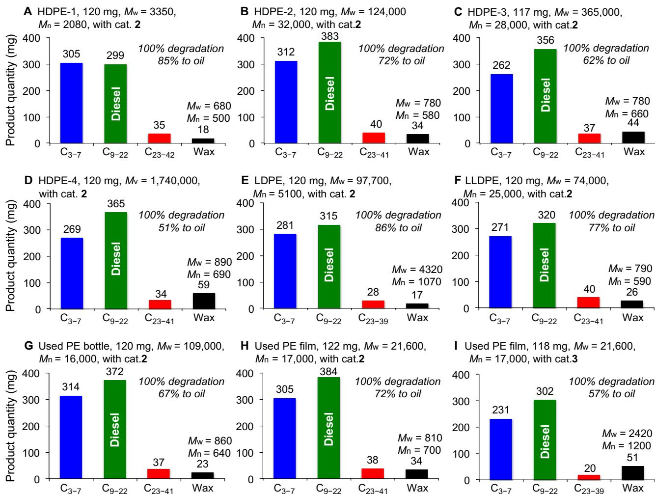
**Fig. 2.** Degradation of various grades of PEs with *n*-octane (2.5 ml for HDPE-1 and LLDPE and 4 ml for all other PEs) by 2 ( $4.2 \mu\text{mol Ir}$ ) and  $\text{Re}_2\text{O}_7/\gamma\text{-Al}_2\text{O}_3$  ( $57 \mu\text{mol Re}_2\text{O}_7$ ): The distribution of degradation products after 4 days at  $175^\circ\text{C}$ . More detailed degradation product distributions are summarized in table S1.
