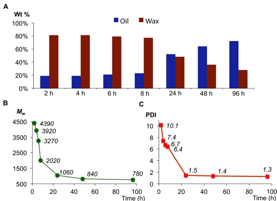
**Fig. 4. Degradation of HDPE-2 (120 to 135 mg) with *n*-octane (4 ml) by **2** (4.2  $\mu$ mol Ir) and  $\text{Re}_2\text{O}_7/\gamma\text{-Al}_2\text{O}_3$  (57.0  $\mu$ mol  $\text{Re}_2\text{O}_7$ ) at 175 °C after 2, 4, 6, 8, 24, 48, and 96 hours. (A) Distributions (wt %) of oil and wax products. (B)  $M_w$  of the isolated PE wax products. (C) Molecular weight distributions (PDI) of the isolated PE wax products.**
