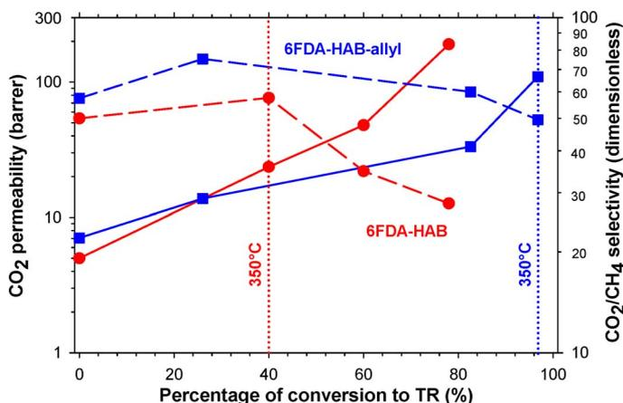
**Fig. 5. Evaluation of the  $\text{CO}_2/\text{CH}_4$  separation properties as a function of the degree of conversion.** Continuous lines represent the evolution of the  $\text{CO}_2$  permeability and dashed lines represent  $\text{CO}_2/\text{CH}_4$  selectivity. Vertical dotted lines denote the results at the same treatment temperature for the CTR polymer (squares) and the classical TR polymer (circles).
