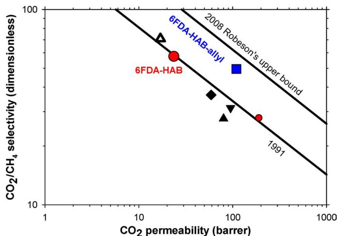
**Fig. 6. Robeson's trade-off for the  $\text{CO}_2/\text{CH}_4$  gas pair.** Samples are represented by symbols as follows: circles for 6FDA-HAB; squares for 6FDA-HAB-allyl; and diamonds (17), triangles pointing down (29), and triangles pointing up (28) for literature data on the polymer 6FDA-HAB synthesized under the same conditions. The largest symbols are for samples thermally treated at 350°C, and small symbols are for the samples thermally treated at 450°C.
