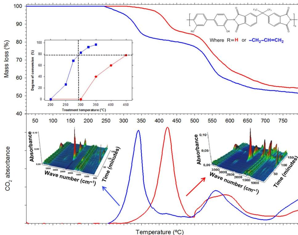
**Fig. 2.** Mass loss and absorbance spectra of CO<sub>2</sub> as a function of temperature for the pristine and allyl-functionalized 6FDA-HAB polymers.
