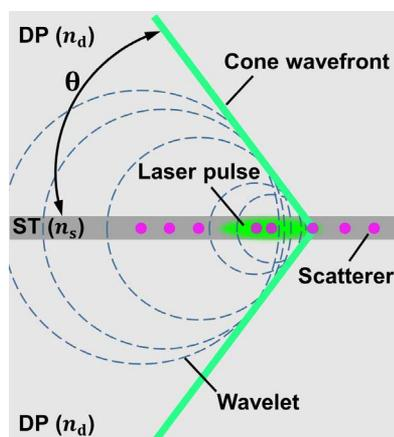
**Fig. 1. Schematic of the thin scattering plate assembly.** The instantaneous light-scattering pattern represents a photonic Mach cone when  $n_s < n_d$ .  $\theta$ , semivertex angle of the photonic Mach cone; DP, display panel; ST, source tunnel;  $n_d$ , refractive index of the display panel medium;  $n_s$ , refractive index of the source tunnel medium.
