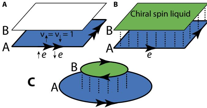
**Fig. 1. Example and phenomenology of topological bootstrap.** (A) Two decoupled layers: a Chern insulator (blue, A) and a free layer of spins (white, B). *e*, electron. (B) After Kondo coupling, the Chern insulator induces a CSL (green) with the opposite chirality. The counterpropagating spin modes gap out, leaving a charge mode. (C) In a terrace construction, the induced and original edge modes are widely separated and coexist.
