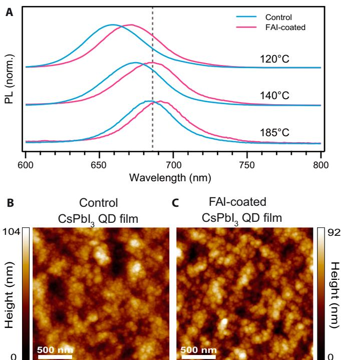
**Fig. 3. Confinement in FAI-coated films.** (A) Normalized (norm.) PL of  $\text{CsPbI}_3$  QD films fabricated with three different sizes (as indicated by the injection temperature during synthesis) of QDs with (pink) and without (blue) FAI treatment. (B and C) AFM images of  $\text{CsPbI}_3$  QD films (B) without and (C) with an FAI posttreatment.
