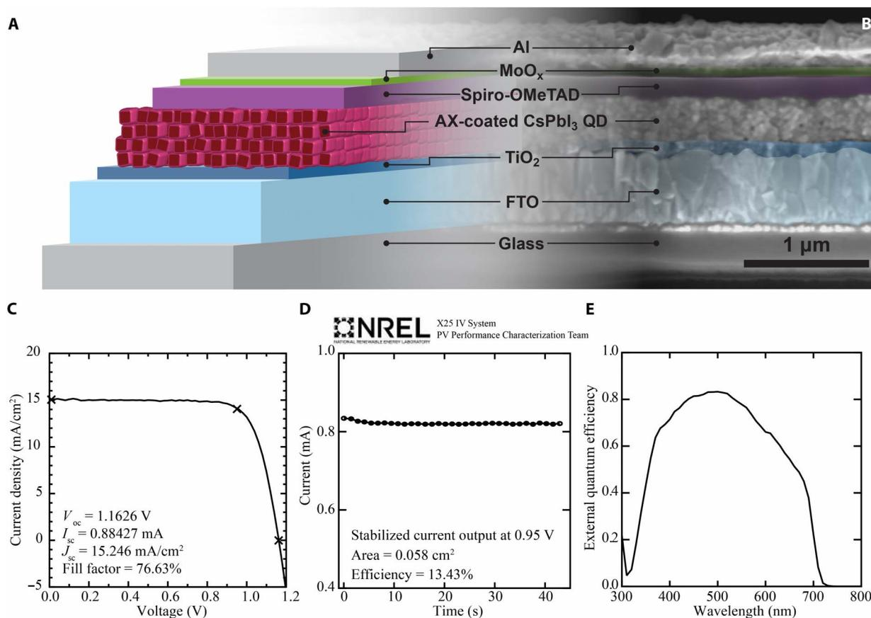
**Fig. 1. High-efficiency FAI-coated CsPbI<sub>3</sub> QDSCs.** (A) Schematic cross section of a solar cell. FTO, fluorine-doped tin oxide. (B) SEM image of a device cross section. (C to E) NREL-certified (C) *J*-*V* characteristics from forward bias to reverse bias, (D) stabilized current at a constant voltage of 0.95 V, and (E) EQE.
