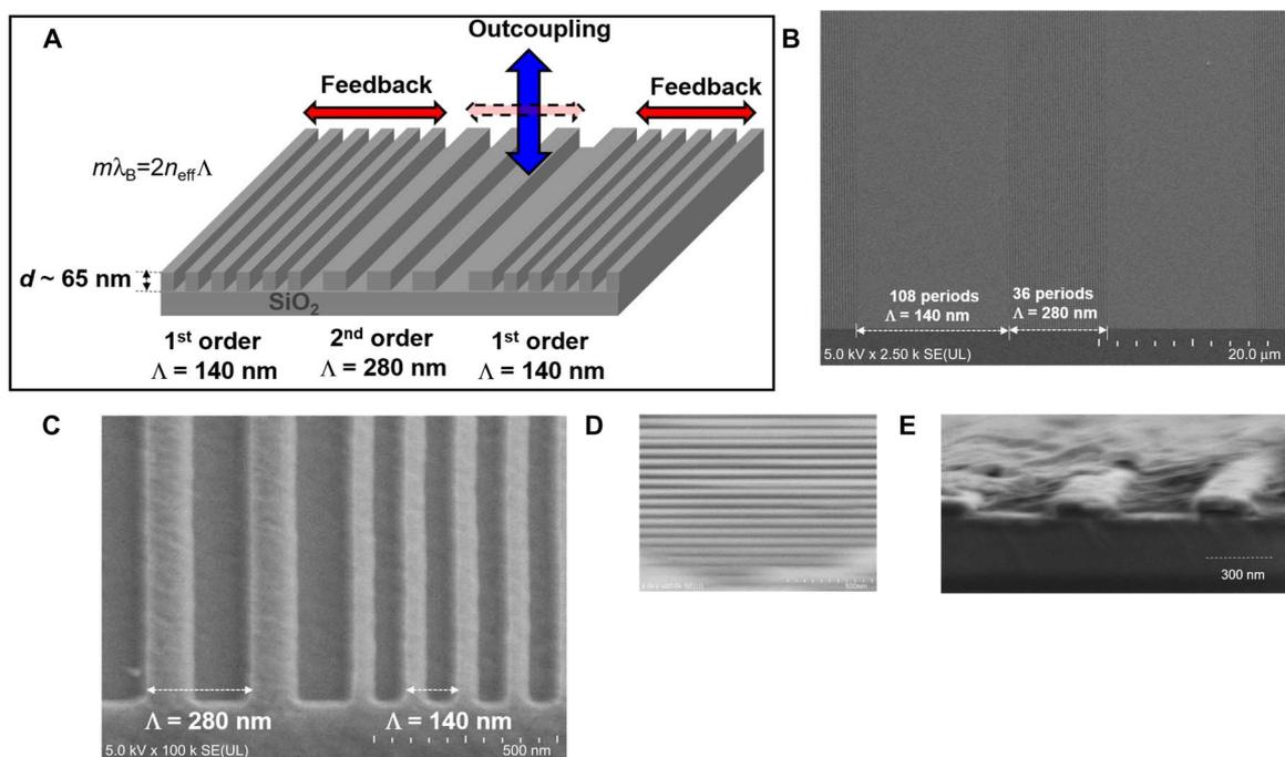
**Fig. 2. Structure of the mixed-order DFB resonators.** (A) Schematic representation of the mixed-order DFB grating structure used in this study. SEM images with (B)  $\times 2500$  and (C)  $\times 100,000$  magnification and (D) SEM image and (E) cross-sectional SEM image of the device after the deposition of a 200-nm-thick BSBCz:CBP blend film.
