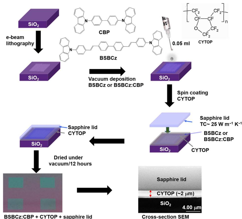
**Fig. 1. Fabrication method of the organic semiconductor DFB lasers.** Schematic representation of the method used to fabricate the organic DFB lasers. The different successive steps involve the fabrication of the DFB resonator structure by electron beam (e-beam) lithography, thermal evaporation of the organic semiconductor thin film, and spin coating of CYTOP polymer film followed by device sealing with a high-thermal conductivity (TC) sapphire lid.
