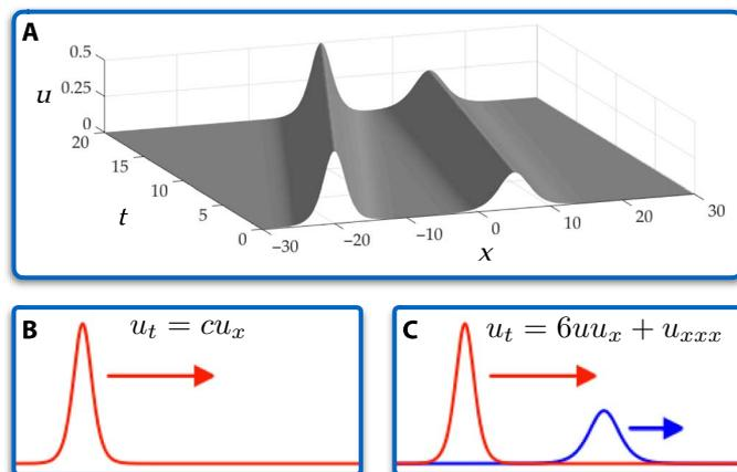
**Fig. 3. Inferring nonlinearity via observing solutions at multiple amplitudes.** (A) Example two-soliton solution to the KdV equation. (B) Applying our method to a single soliton solution determines that it solves the standard advection equation. (C) Looking at two completely separate solutions reveals nonlinearity.
