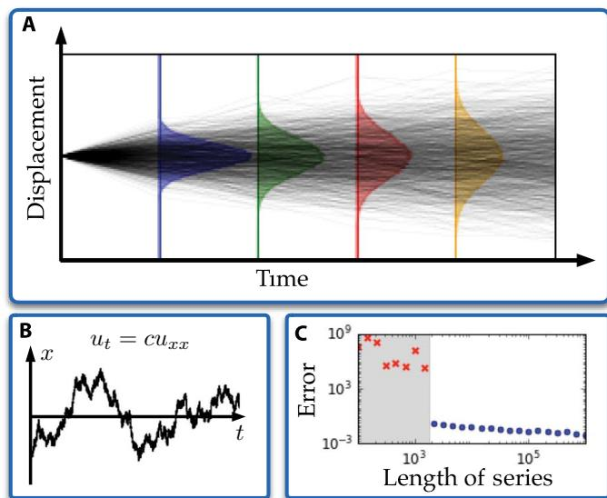
**Fig. 2. Inferring the diffusion equation from a single Brownian motion.** (A) Time series is broken into many short random walks that are used to construct histograms of the displacement. (B) Brownian motion trajectory following the diffusion equation. (C) Parameter error ( $\|\xi - \xi^* \|_1$ ) versus length of known time series. Blue symbols correspond to correct identification of the structure of the diffusion model  $u_t = cu_{xx}$ .
