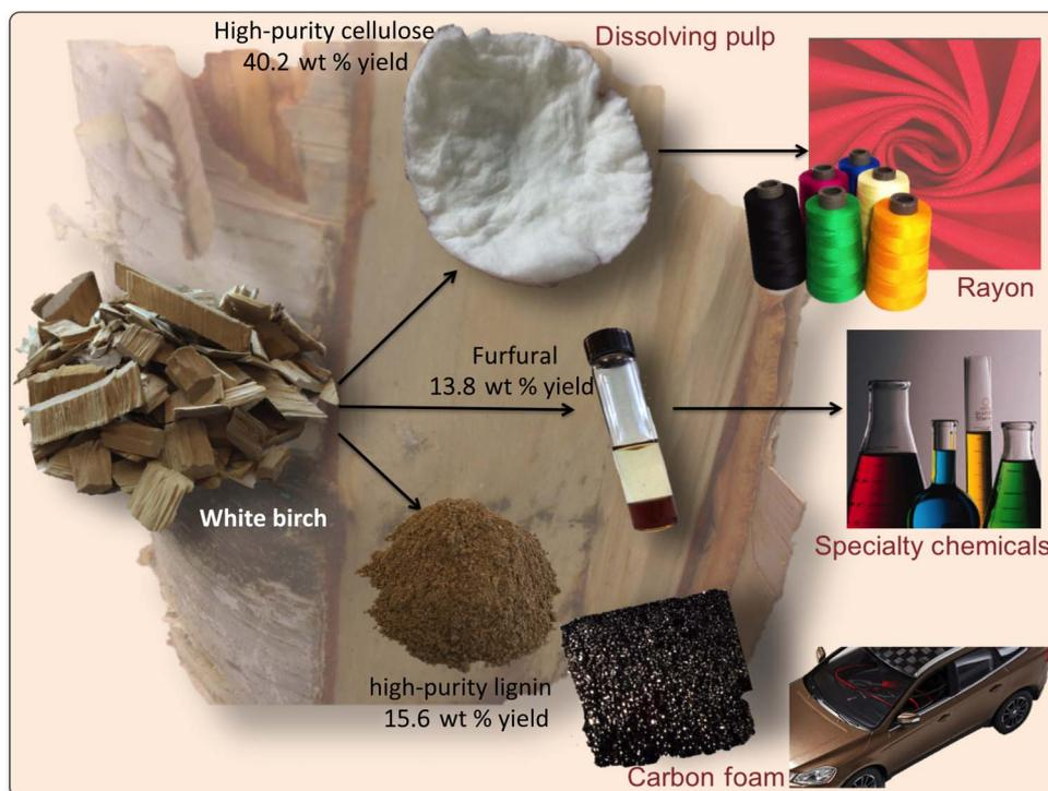
**Fig. 1. TriVersa Process.** Lignocellulosic biomass can be fractionated into its main components to replace petroleum-derived chemicals used in daily life. Initial composition of white birch (dry weight): hexosan, 45.0 wt %; pentosan, 25.3 wt %; lignin, 21.7 wt %. The yields have been calculated on the basis of our techno-economic analysis.
