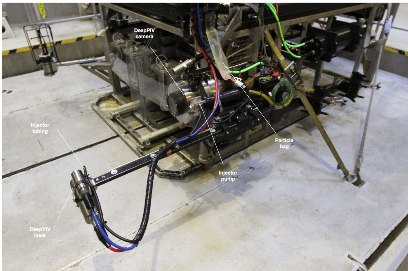
**Fig. 1.** Experiments were conducted on board R/V *Western Flyer* using DeepPIV's particle injector deployed from ROV *Doc Ricketts*. We conducted in situ feeding studies of giant larvaceans using a modified dye injector pump developed with the DeepPIV hardware (20). A peristaltic injector pump emptied a bag filled with microplastic particles and dispensed particle-rich fluid through the tubing nearby an animal.
