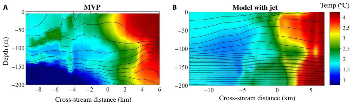
**Fig. 4. Average temperature and density sections.** (A) Composite temperature (color) and density (black contours), averaged for all MVP sections. (B) Along-stream ( $x$ ) averaged temperature (color) and density (black contours) from the model with the ACC jet at 53 days. The initial temperature was independent of depth in the model.
