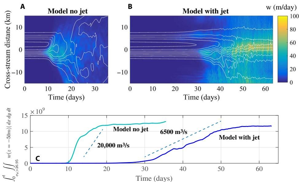
**Fig. 5. Vertical velocity and subduction.** rms vertical velocity at  $z = 50$  m depth with respect to an average in the  $x$  direction, from the model without (A) and with (B) the ACC jet. White contour lines show  $x$ -averaged density with a contour interval of  $0.01 \text{ kg m}^{-3}$ . Volume of water with potential density  $\sigma_\theta > 26.95 \text{ kg/m}^3$  subducted below  $z = -50$  m. The slope of the dashed lines corresponds to the labeled volumetric subduction rate.
