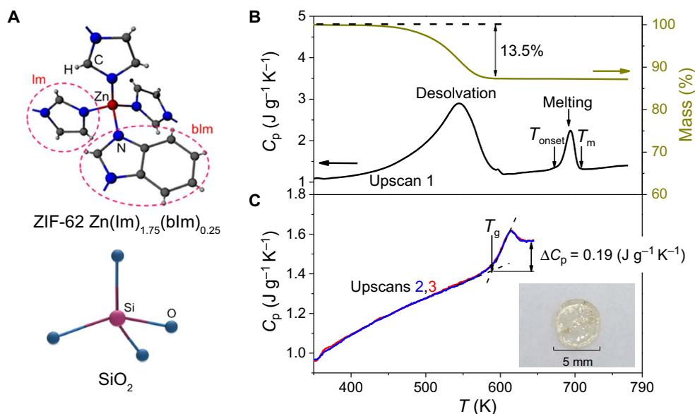
**Fig. 1. Structural units and calorimetry of ZIF-62.** (A) Similarity between tetrahedra in silicate glasses and ZIF-62 lm/blm networks. (B)  $C_p$  and mass loss versus  $T$ , heated at  $10 \text{ K min}^{-1}$ , following desolvation to eventual melting at  $T_m = 708 \text{ K}$ . (C)  $C_p$  upscans of ZIF-62 glass quenched from above  $T_m$  showing a clear glass transition ( $T_g = 595 \text{ K}$ ), yielding  $T_g/T_m$  (0.84). Inset: Optical image of a transparent MQ glass.
