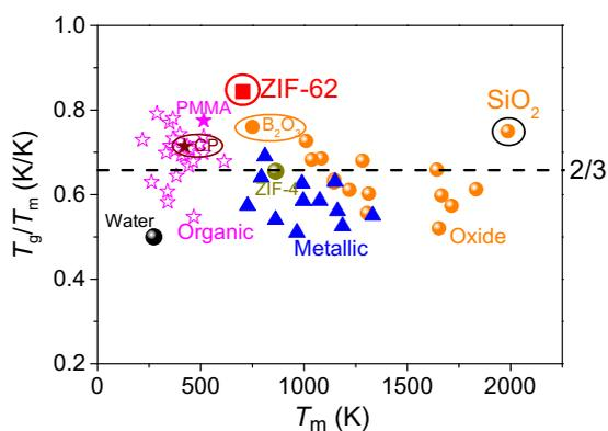
**Fig. 4. The ultrahigh  $T_g/T_m$  ratio of ZIF-62.** The comparison in  $T_g/T_m$  ratio between ZIF-62 and other types of glass-forming systems, including water (29, 30), oxide (33), metallic (34), and organic (35, 36)—good GFA typified by CPs, PMMA, B $_2$ O $_3$ , and SiO $_2$  in contrast with the ultrahigh GFA of the ZIF-62.
