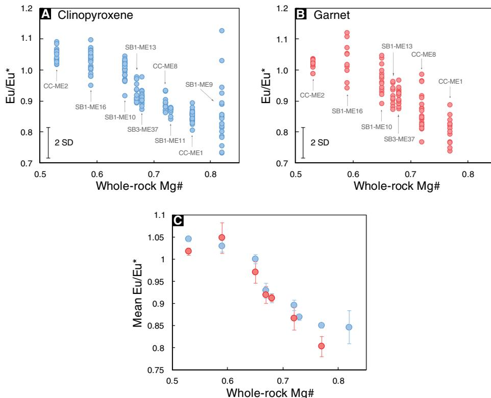
**Fig. 1. Eu/Eu\* in clinopyroxene and garnet in deep arc cumulates as a function of whole-rock Mg#.** (A and B) Individual spot data measured by laser ablation ICP-MS. The error bars denoted in (A) and (B) are the long-term (~8 months) reproducibilities (2 SD) of measuring Eu/Eu\* in basaltic glass standards BIR-1G and BCR-2G. (C) The mean Eu/Eu\* in clinopyroxene and garnet for each rock sample. Error bars are 2 standard error of mean (2 SEM).
