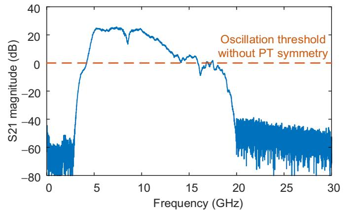
**Fig. 3. S21 magnitude response of the OEO with only one loop closed.** It is measured by a vector network analyzer (VNA) connected between the MZM and the EA with the measurement direction indicated in Fig. 1.
