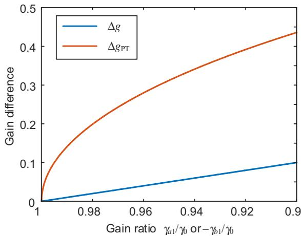
**Fig. 2. Gain difference enhancement with PT symmetry.** The gain difference between the oscillating mode and the secondary mode within a regular single-loop OEO (blue) and a PT-symmetric OEO (red) is illustrated for comparison.
