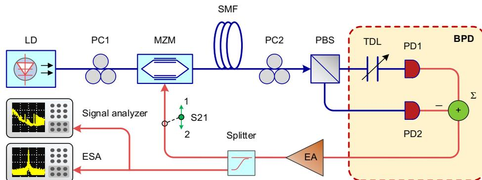
**Fig. 1. Block diagram of the PT-symmetric OEO.** LD, laser diode; PC, polarization controller; MZM, Mach-Zehnder modulator, SMF, single-mode fiber; PBS, polarization beam splitter;  $\Sigma$ , microwave combiner; EA, electrical amplifier; ESA, electrical spectrum analyzer.
