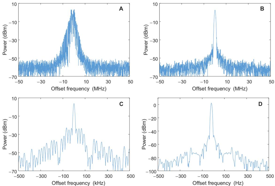
**Fig. 4. The electrical spectra of the microwave signals generated by the PT-symmetric OEO.** The spectra are measured at a central frequency at 9.867 GHz. (A) Multimode oscillation measured with a resolution bandwidth (RBW) of 3 MHz. (B) Single-mode oscillation measured with an RBW of 3 MHz. (C) Single-mode oscillation measured with an RBW of 9.1 kHz. (D) Single-mode oscillation measured with an RBW of 9 Hz.
