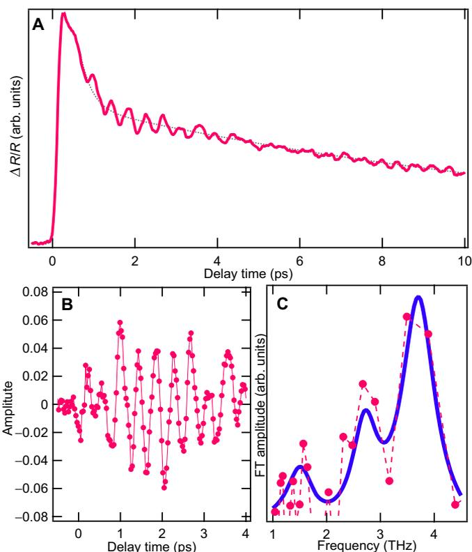
**Fig. 4. Dynamics of the differential reflectivity change.** (A) Transient reflectivity: relative intensity changes from a bulk sample at the LT phase  $\sim 200$  K recorded at the excitation wavelength (800 nm, 100 fs) and fluence (1 mJ/cm<sup>2</sup>). (B) Subtraction from the fitting curve to raw data of (A). (C) FTs of the transient reflectivity of (B). Dots are the result, and a curve as a guide to the eye is the fit of Lorentzians.
