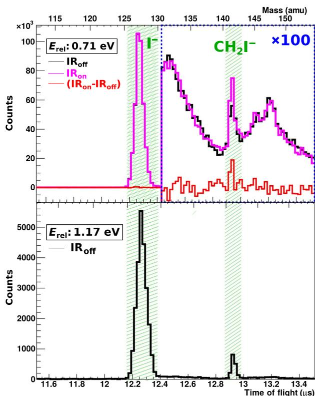
**Fig. 2.** Time-of-flight traces of the reaction products of the  $\text{F}^- + \text{CH}_3\text{I}$  reaction for two different relative collision energies. The conversion to atomic mass units (amu) is plotted on the upper horizontal axis. At the lower collision energy, we performed every other ion-molecule crossing with the infrared excitation laser present. The difference signal is plotted in red.
