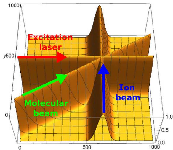
**Fig. 3.** Illustration of the overlap of the molecular beam, ion beam, and laser beams in the center of the velocity map imaging spectrometer. From the overlap integral, we determined the excited fraction of the neutral molecules in the reaction volume.
